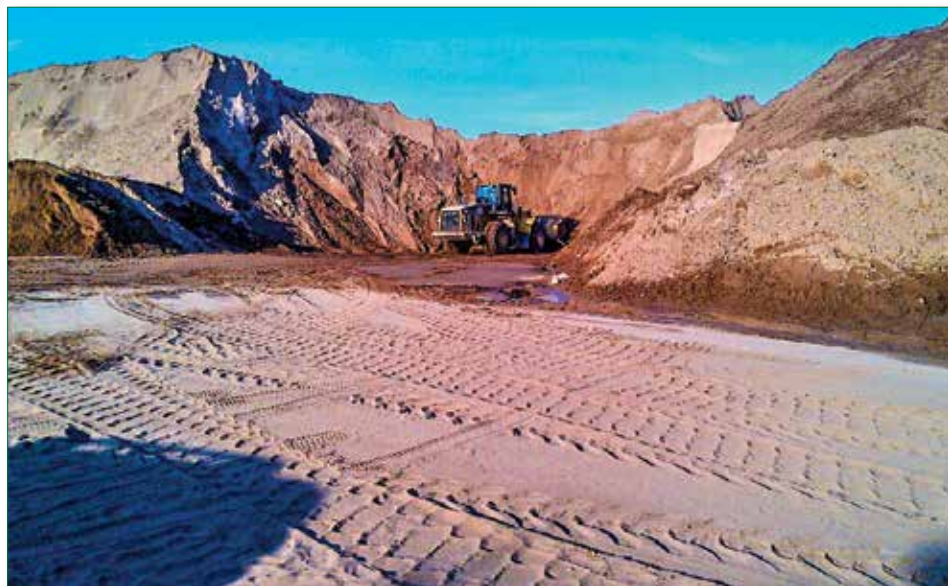
Clean sand that has been hydraulically separated at the Erie Pier CDF and is now ready for beneficial reuse for construction and industrial use (U.S. Army Corps of Engineers, Detroit District photo).
