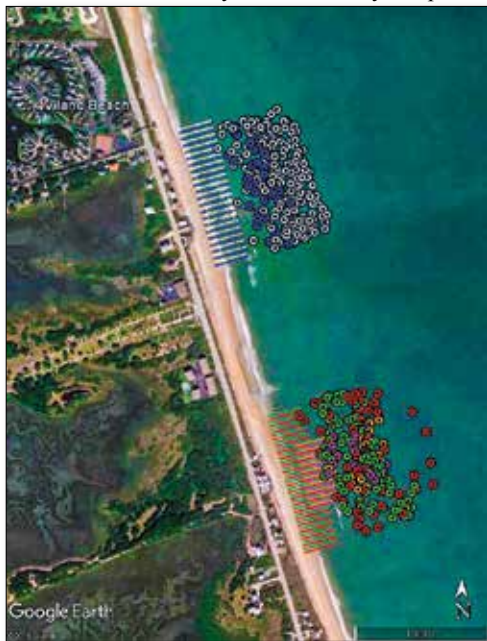
Figure 2. Two near-shore berms were designed: northern berm as an elongated bar and the southern berm as mound shaped. The colored lines are the vessel heading line for placement and the circles show the actual hopper placement locations. The dredge was instructed to place the sediment as close to the shoreline as possible given the tide.
