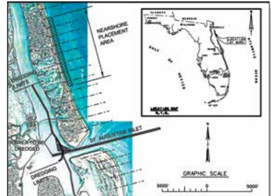
Figure 1. Near-shore berm project location at Vilano Beach, FL, north of St. Augustine Inlet, with the permitted dredging and near-shore placement areas shown. The near-shore berm placement in this study occurred in two sections of the larger box shown here.
