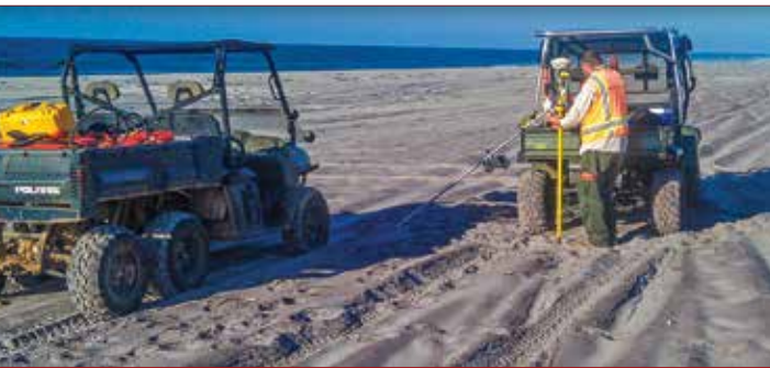
McKim & Creed field crews collected blind checkpoints at the site to independently verify the accuracy of the UAS data.
