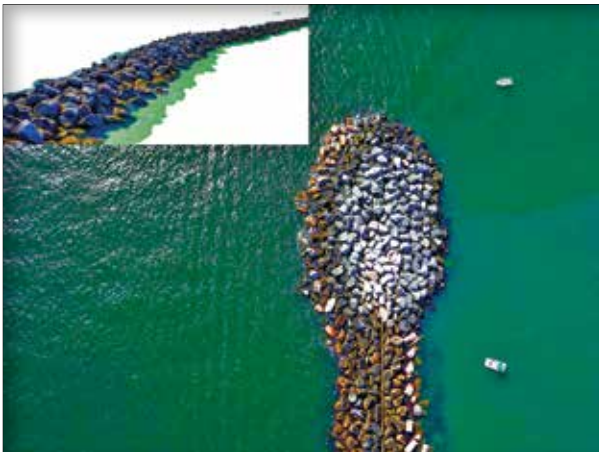
The test site included two rock jetties. The inset is the 3D model produced from the UAS data, and the background image is a photo of the jetty taken by the drone.
