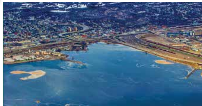
Shown 21st Ave West Embayment with two shoal features that are currently sticking out of the water. The vast majority of the 600,000 yd 3 of dredged material placed in this area is underwater (U.S. Army Corps of Engineers, Detroit District photo).
