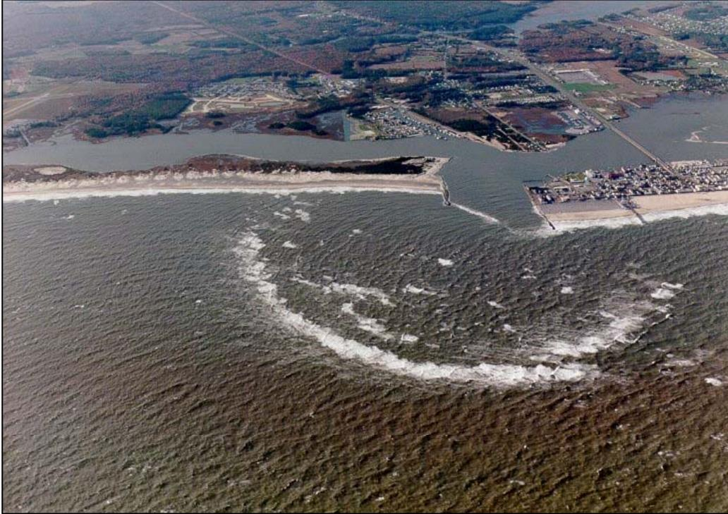
**FIG. 2. Pattern of Wave Breaking on the Ebb Shoal and Bar, Ocean City Inlet, Maryland.
