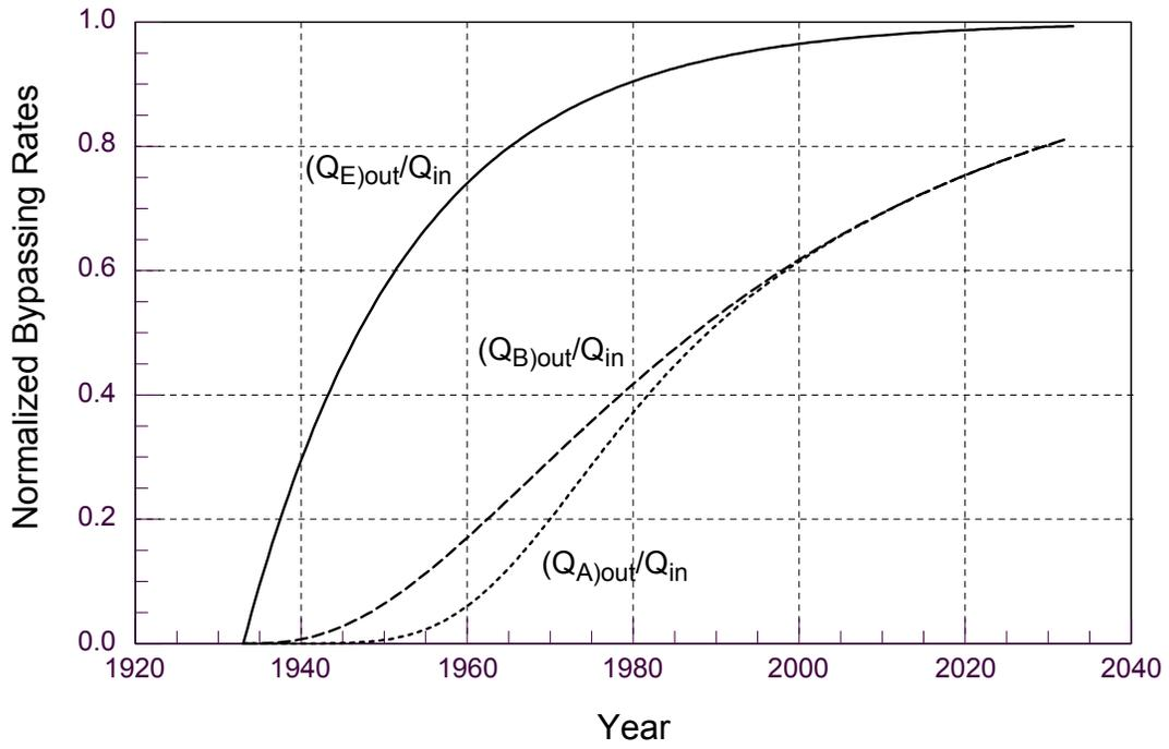
FIG. 7. Calculated Bypassing Rates, Ocean City Inlet
