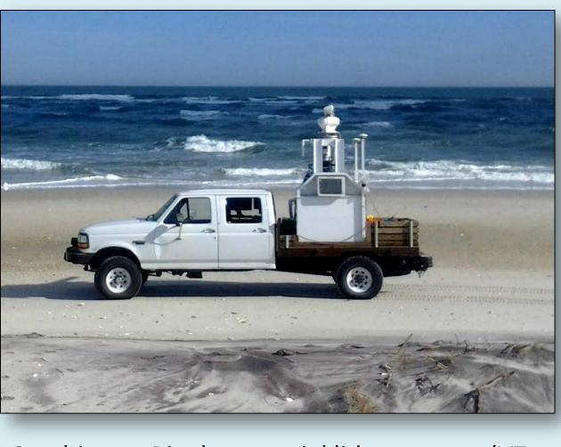
Combines a Riegl terrestrial lidar scanner (VZ-1000), Applanix POS-LV, and X-Band Radar to map beach topography and surf-zone waves
