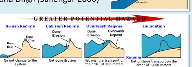
2. Simple Dune Erosion Models - Relate volume of erosion through time to the momentum flux from wave impact (e.g. Larson et al., 2004; Palmsten & Holman, 2012)
