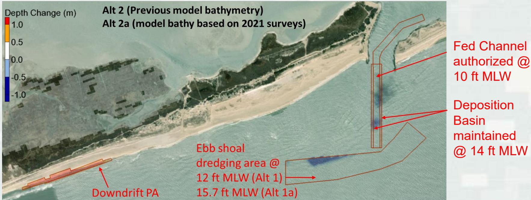
Removal of 17,000 cubic m from channel and deposition basins
