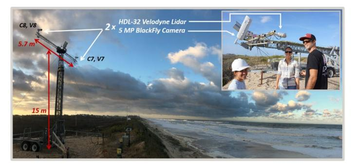
Collected 2Hz imagery 10 min every hour concurrent with in-situ pressure sensors
