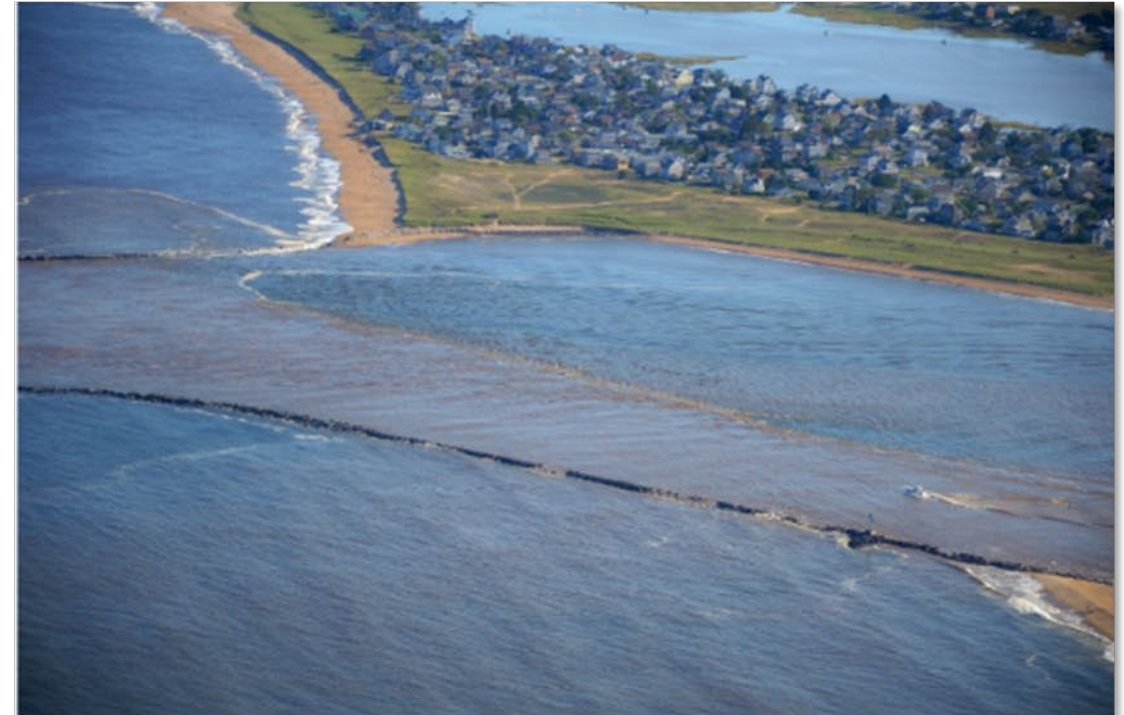
Sediment plume ebbing through Merrimack River Inlet in 2011. Note the stagnant water along Reservation Terrace at the top of the photo. The coloration also indicates a lack of mixing between the outward flow and the waters beyond the navigation channel. (DCR, 2021)
