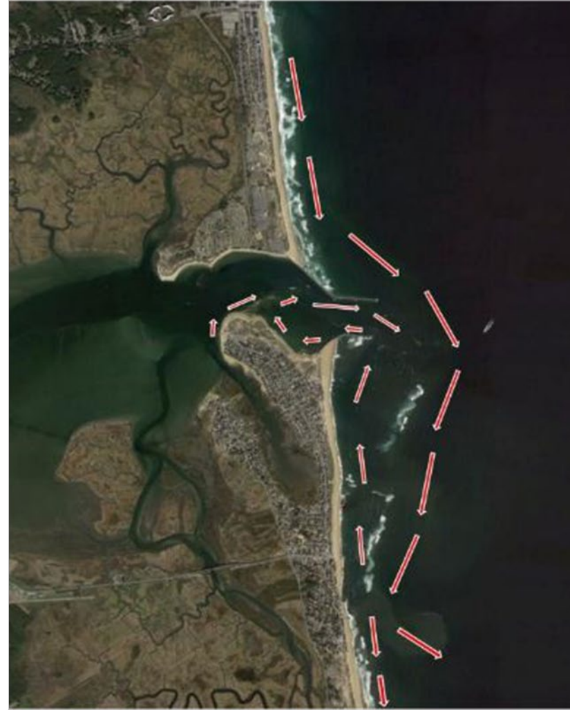
Sediment transport patterns based on modeled flow patterns, imagery, and existing literature. (DCR, 2021)
