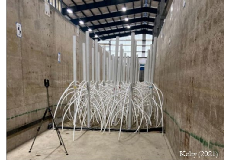
Kelty prototype-scale mangroves made of PVC. Oregon State University
