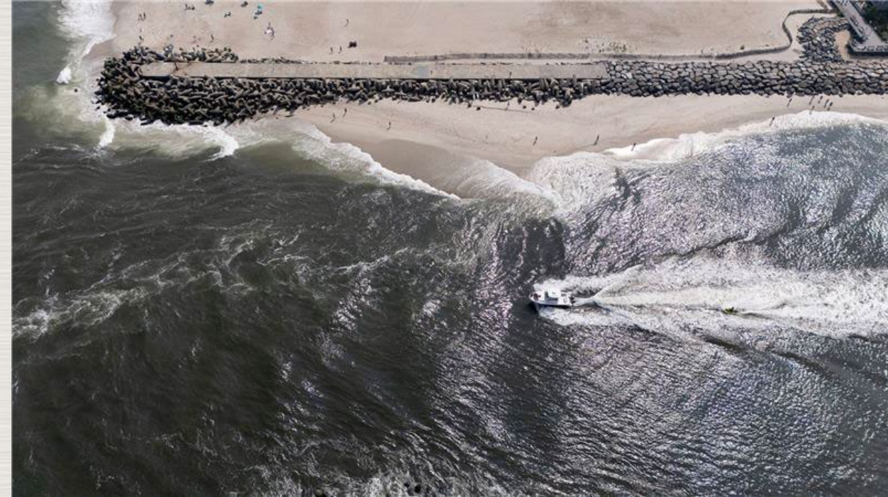
Severe shoaling in the navigation channel of Manasquan Inlet NJ
