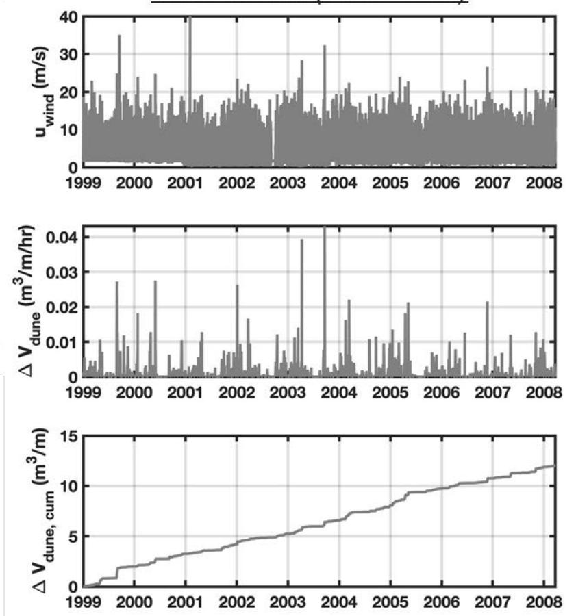
AeoliS can provide all inputs GENCADE needs to account for sediment losses/gains to dune from aeolian and marine processes. Closely matches rates found from field.
