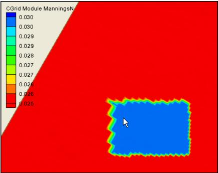
Figure 19. Contoured display of bottom friction values.
