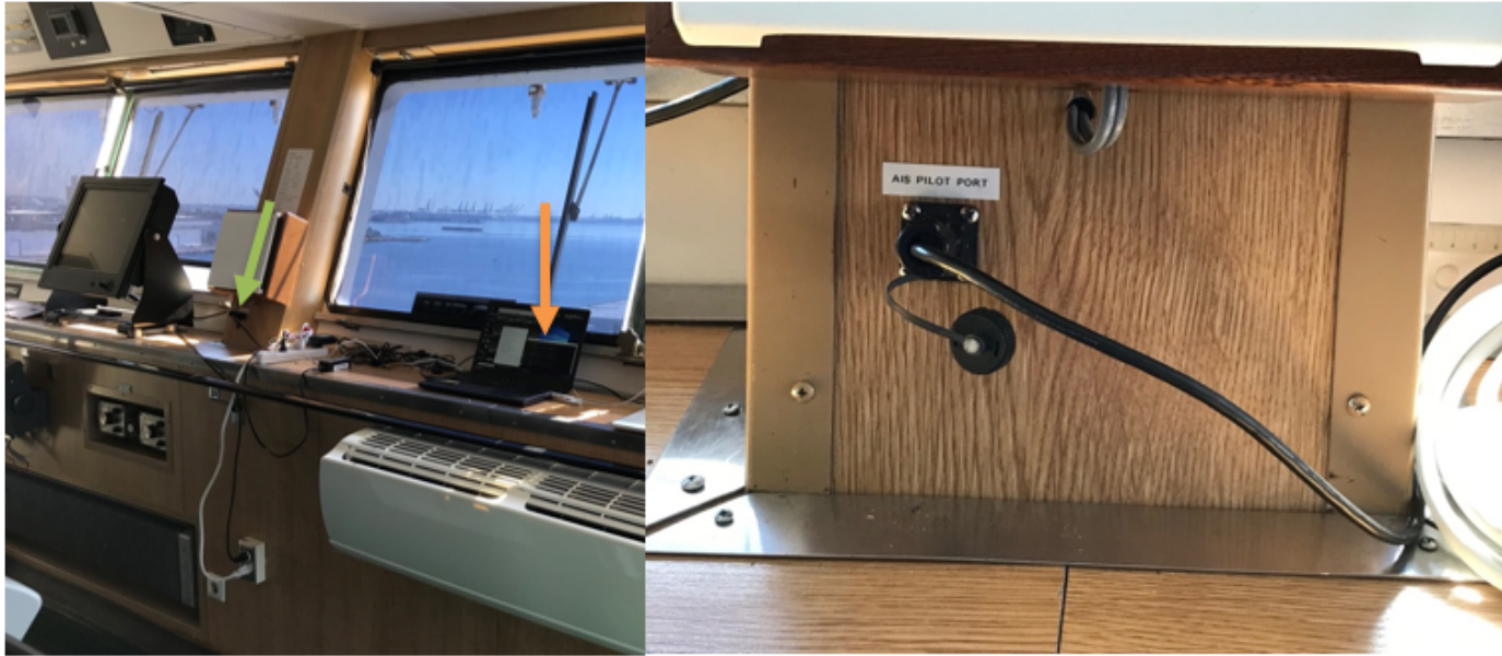
Figure 7. Left: Laptop (orange arrow) on ledge to the right of the pilot port (green arrow). Right: close-up of pilot port.
